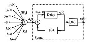
Figure 1 Analog computer concept for the chaotic neuron circuit. The nonlinear block is given by  $g(x) = kx - \alpha f(x)$ , according to (1).
