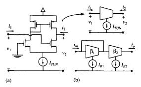
Figure 4 (a)Tunable transconductor. (b) Programmable current mirror.
