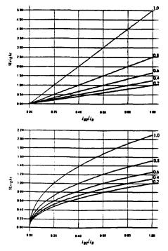
Figure 5 Weight  $(i_{\sigma}/i_{in})$  variation with  $I_{B2}/I_B$  for different values of  $I_{B1}/I_B$  in Fig. 4(b). (a) Transconductors operating in weak inversion,  $I_B = 10$ nA.
