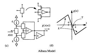
Figure 3 Piecewise linear mapping circuits for the neurons.
