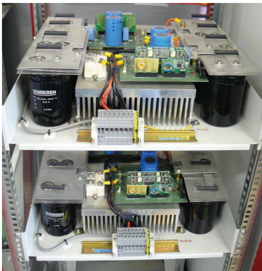
Fig. 8. 5 kVA single-phase two-cell SDC-CHB prototype.
