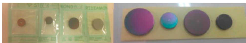
Figure 1. On the left are samples without a TiO 2 film and on the right, samples with TiO 2 .
