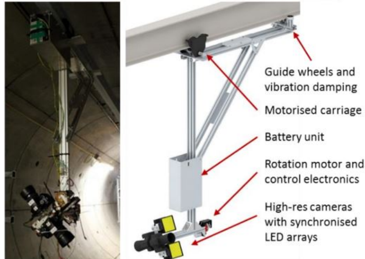
Figure 5: Tunnel reconstruction prototype (Stent et al., 2015).
