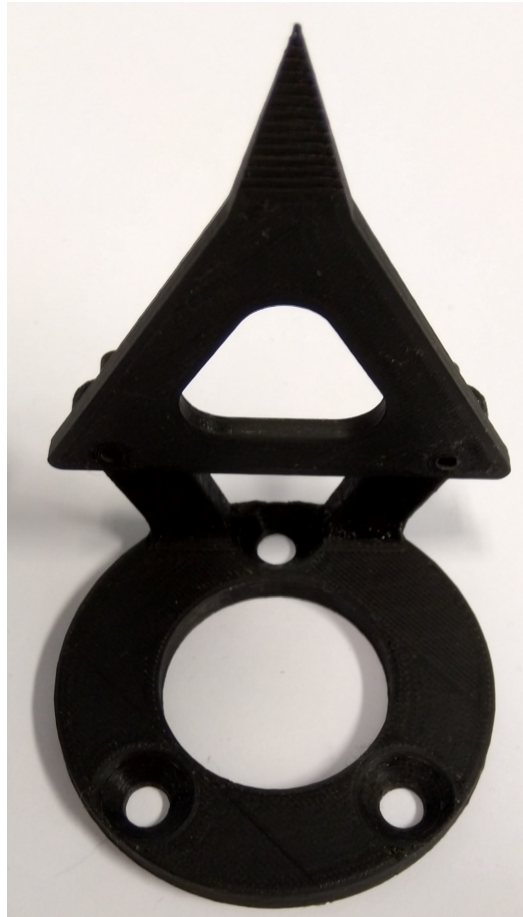
Figure 16: 3D printed accessory to support the Intel RGBD camera and a sharp tool mounted on it to obtain points in Robot coordinates.
