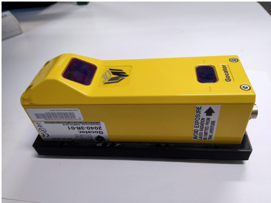
Figure 14: Gocator 2040 in its 3D printed support.
