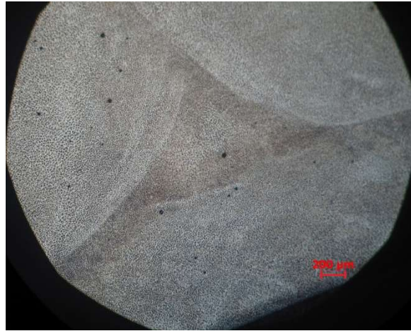
Figure 40 - Layer disposition, with evidence of possible gap formation on component P2.
