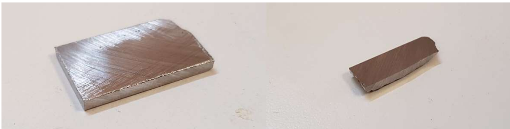
Figure 29 - Detail of the small pieces cut from components W2 (on the left) and P2 (on the right) for the optical microscopy test.
