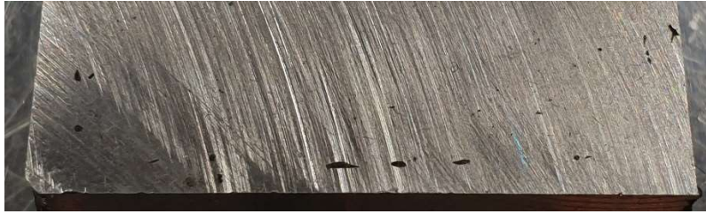
Figure 38 - Identifiable gaps on component W2, after performing a horizontal cut.
