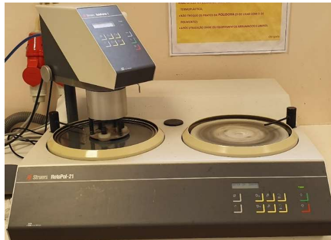
Figure 22 - The Struers RotoPol-21 equipment, the polishing machine used to prepare the components for microhardness testing.
