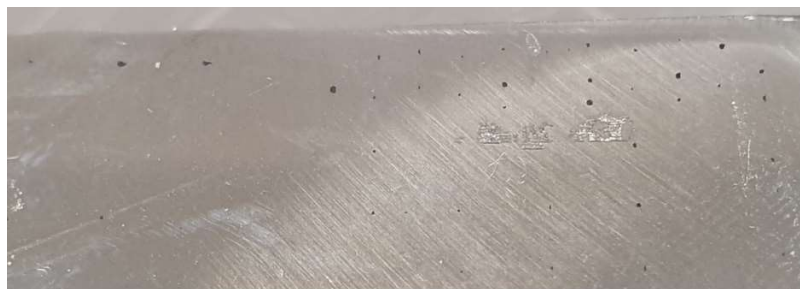
Figure 37 - Identifiable gaps on component W2, after performing a vertical cut.
