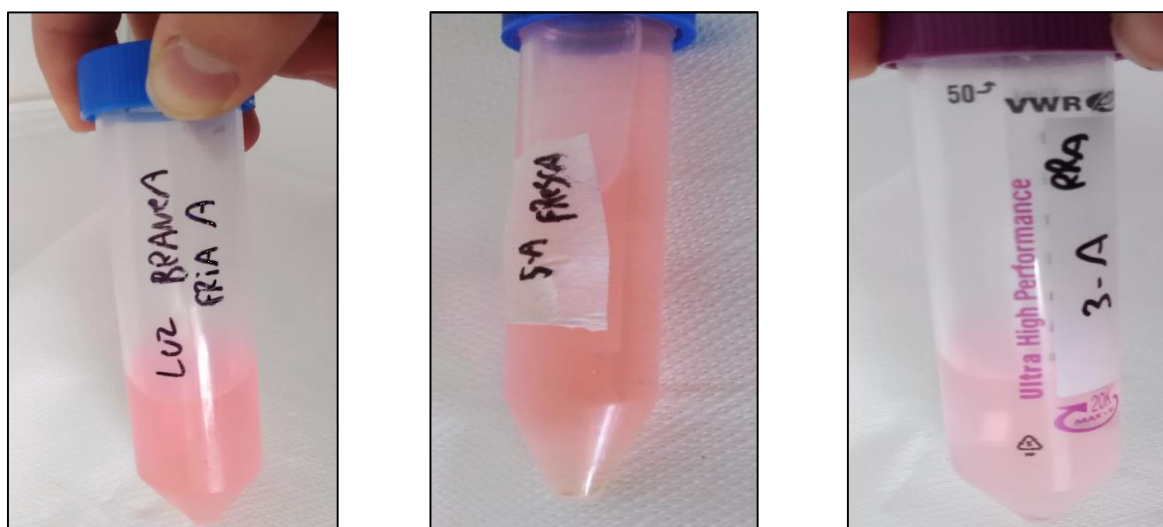
Figure 4.15: Photographs illustrating the visual aspect of the R-PE and R-PC-containing supernatants resultant from the mechanical extraction of PBPs with the tissue homogenizer applied to G. gracilis culture samples; from left to right, the assays “Cool White Fluorescent” (CWF), “Ammonium, Phosphate & Light Increase” and “Control”, respectively, from the Independent and 3 rd Set of Independent Trials.
