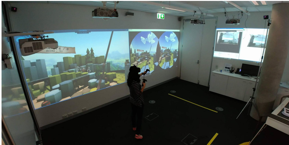
Fig. 4.2.: VR game studio room set up with a play area of 2.5 x 3.5 metres, marked with yellow tape.
