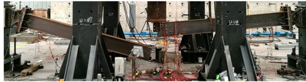
Specimen S4: fracture of bolts on the LHS
