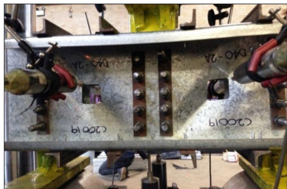
Fig 2.24: Shear failure mode with square web holes by C.H. Pham et al. [21]
