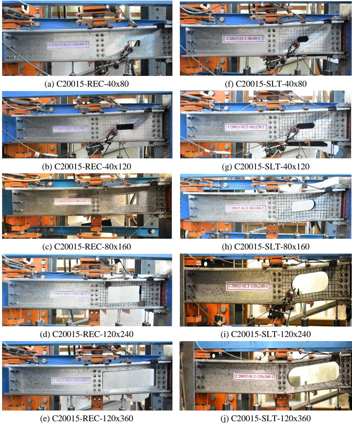
Fig 3.11: Failure modes in the shear tests with rectangular and slotted web openings
