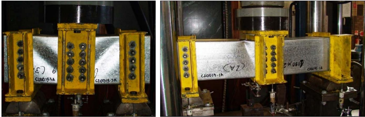
(a) Failure mode of predominantly shear test ( AR = 1.0 ) (b) Failure mode of combined shear and bending test ( AR = 2.0 )
