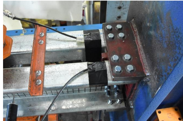
Fig 3.6: Arrangement of inclinometers
