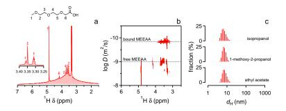
**Figure 5.2:** (a) 1D <sup>1</sup>H NMR of Cu NCs after ligand exchange to MEEAA and dispersed in methanol- $d_4$ . (b) DOSY spectra of the same Cu NCs dispersion. (c) Hydrodynamic diameter distribution by Dynamic light scattering (DLS) of Cu NCs capped with MEEAA in different solvents. Labeled resonances are identified as (1-6) MEEAA resonances, (‡) methanol and (†) residual methanol- $d_4$ .
