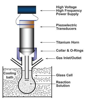
**Figure 2.2:** Schematic representation of a typical laboratory rig for sonochemical reactions using a high intensity ultrasonic horn. Reprinted from reference<sup>49</sup>
