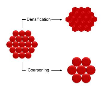
**Figure 5.1:** Graphical representation of an arrangement of particles undergoing densification and coarsening, the two basic phenomena that lead to sintering.
