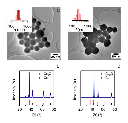
Figure 3.1: Low-resolution, brightfield TEM image of Cu NCs formed by a 2 g/L, 2:1 oleylamine:  $Cu(HCO_2)_2$  synthesis under (a) ambient and (b) nitrogen atmosphere; (insets) Size histograms determined based on the analysis of 200 NCs in TEM images. XRD pattern of pristine NCs synthesized under (c) ambient and (d) nitrogen atmosphere. The mixture for the synthesis under nitrogen was degassed prior to the reaction.
