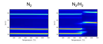
Figure A.8: In-situ XRD plot of comercial CuO heated up under different atmospheres ( $N_2$  and  $N_2 : H_2$ .)
