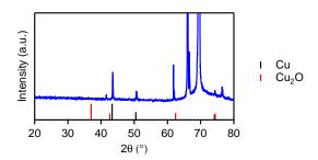
Figure A.9: XRD plot of as-synthesized Cu NCs described in Figure 5.6b.
