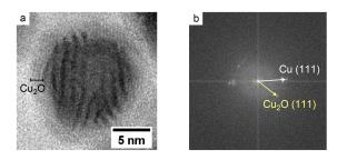
Figure A.10: (a) High-resolution, brightfield TEM image of Cu NCs synthesized in an open atmosphere 2 weeks before the imaging. The reagents concentrations were set at:  $0.63M \operatorname{Cu(HCO_2)_2}$  and  $1.26M \operatorname{OlNH_2}$ . The synthesis proceeded with a heating rate of  $10^{\circ}\mathrm{C/min}$ . until  $140^{\circ}\mathrm{C}$  and then held at this temperature for 10 min. (b) Fast Fourier Transform of image (a), showing their indexed lattice planes.
