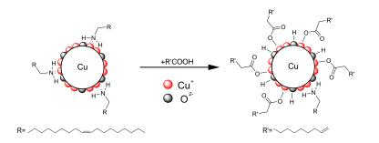
**Figure 4.10:** Surface chemistry model of the Cu NCs before and after addition of a carboxylic acid. The binding of the carboxylate to the metal is indicative and not meant to represent a specific binding mode.
