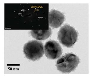
Figure 2.5: Transmission electron microscopy image showing the  $Cu/Cu(HCO_2)_2$  core-shell particles. Inset: selected area electron diffraction pattern of a high resolution image showing the presence of crystalline  $Cu(HCO_2)_2$ . Reprinted from reference<sup>59</sup>
