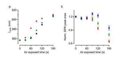
**Figure 5.3:** (a) Peak wavelength and (b) peak area of the surface plasmon resonance after starting the permanent exposure of a dispersion of Cu NCs to air. The different data sets pertain to Cu NCs capped by (red circles)  $OlNH_2$ , (blue squares) UDA, and (green triangles) oleic acid.
