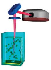
**Figure 2.3:** Schematic representation of a laboratory experimental set-up for a laser ablation system in solvent. Reprinted from reference<sup>64</sup>
