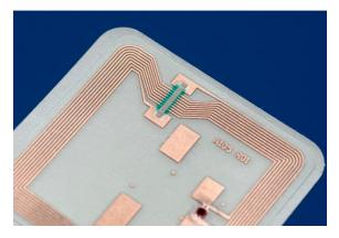
Figure 1.1: Printed RFID tag (Reprinted from reference.<sup>10</sup>)
