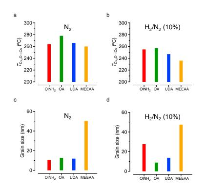
**Figure 5.5:** (a-b) Transition temperature characterizing the reduction of  $Cu_2O$  NCs to Cu, depending on the ligand and the annealing atmosphere. (c-d) Grain size of the crystallites as obtained from the diffractogram recorded at 300°C, depending on the ligand and annealing atmosphere. Each bar represents a different ligand: (red)  $OlNH_2$ , (green) oleic acid, (blue) UDA and (orange) MEEAA.
