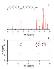
**Figure A.1:** (a) 1D <sup>1</sup>H NMR spectrum of a solution of 10  $\mu$ l of OlNH<sub>2</sub> in toluene-*d*<sub>8</sub>. (b) Correlation Spectroscopy (COSY) spectrum of the same solution.
