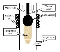
**Figure 2.4:** Schematic representation of the flow-levitation synthesis method for Cu nanoparticles. Reprinted from reference<sup>77</sup>
