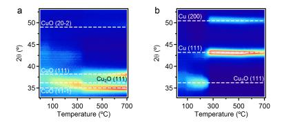
**Figure 5.4:** Contour plots of x-ray diffractograms of films of dropcast, UDA-capped Cu NCs recorded *in-situ* during annealing under ambient (a) and  $N_2$  (b). Equivalent plots of OlNH<sub>2</sub>, oleic acid (OA) and MEEAA-capped Cu NCs are available in the appendix section A.2.3.
