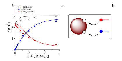
Figure 4.6: (a) Representation of (markers) the experimental titration of  $\rm OlNH_2$ -capped Cu nanocrystals with UDA and (full lines) a simulation of the  $\rm OlNH_2/UDA$  titration assuming competition for homogeneous surface sites. Here, the parameters were set so as the fit the surface concentration of bound UDA. (b) Graphical representation of the homogeneous exchange model.
