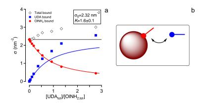
**Figure 4.5:** (a) Representation of (markers) the experimental titration of  $OlNH_2$ -capped Cu nanocrystals with UDA and (full lines) a simulation of the  $OlNH_2/UDA$  titration according to the one-by-one exchange model. The annotation provides the initial surface concentration  $\sigma_0$  of bound  $OlNH_2$  and the equilbrium constant K as determined from a best fit of the surface concentration of bound  $OlNH_2$  to Eq 4.4. (b) Graphical representation of the one-by-one exchange model.
