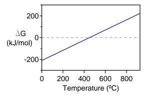
Figure A.6: Ellingham diagram of the reaction A.1 at a  $O_2$  concentration of 1 ppm and a total pressure of 3 mbar.
