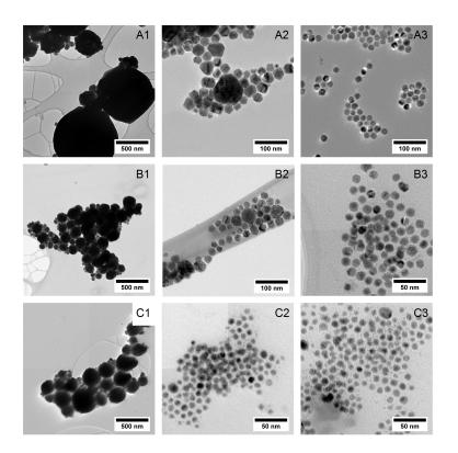
**Figure 3.5:** Low-resolution, brightfield TEM images of Cu NCs synthesized with different concentrations of copper: (A) [Cu]=10 g/L, (B) [Cu]=20 g/L, (C) [Cu]=40 g/L and different molar ratio between  $OlNH_2$  and copper formate: (1)  $OlNH_2:Cu(HCO_2)_2=1:1$ , (2)  $OlNH_2:Cu(HCO_2)_2=2:1$ , (3)  $OlNH_2:Cu(HCO_2)_2=3:1$ .
