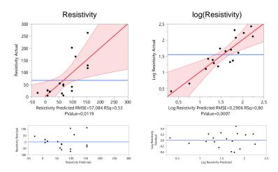
**Figure A.11:** Experimental data versus predicted in the model for both resistivity and log(resistivity), and residuals of the plots.
