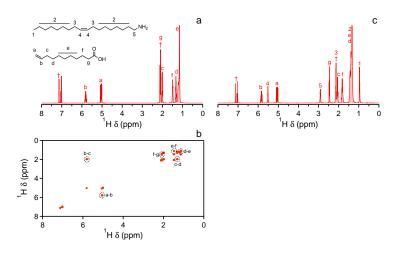
**Figure A.4:** (a) 1D <sup>1</sup>H NMR spectrum of UDA in toluene- $d_8$ . (b) COSY spectrum of UDA in toluene- $d_8$ , in which the different cross peaks have been assigned to couples of neighboring protons. (c) 1D <sup>1</sup>H NMR spectrum of OlNH<sub>2</sub> and UDA in toluene- $d_8$ . Labeled resonances are identified as (1-5) OlNH<sub>2</sub> resonances, (a-g) UDA and (†) toluene- $d_8$ .
