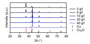
Figure 3.3: XRD patterns of Cu NCs synthesized with different concentrations of Cu without protective atmosphere. The molar ratio of  $OlNH_2:Cu(HCO_2)_2$  has been kept at 2:1 and the heating rate at  $20^{\circ}C/min$  for all syntheses. The NCs were purified and dried in ambient conditions prior to measurement.
