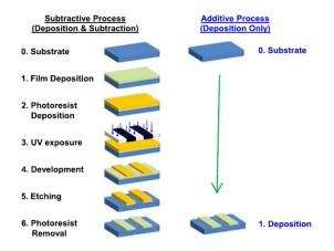
**Figure 1.2:** The traditional photolitography procedure compared to the PE approach for producing RFID antennas. (Reprinted from reference.<sup>18</sup>)
