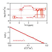
Figure A.3: (top) DOSY spectrum of a dispersion of Cu nanocrystals stabilized by  $OlNH_2$  after 1 hour of air exposure. (bottom) Decay of the intensity of the alkene resonance at 5.5 ppm with increasing field gradient strength. Fitting the decay to a single exponential yields the diffusion coefficient as indicated.
