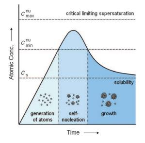
**Figure 2.1:** Schematic representation of the LaMer model in a plot of atomic concentration against time, illustrating the generation of monomer, nucleation, and subsequent growth of colloidal nanoparticles.  $C_{min}^{nu}$  indicates the saturation point for atoms in solution, when nucleation events start to occur.  $C_s$  indicates the equilibrium state reached between the atoms in the nanoparticles and the atoms in solution. Reprinted from reference<sup>22</sup>
