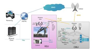
Fig. 2. Smart Highway Architecture
