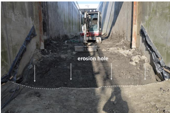
Figure 9 Erosion along the whole width of the Delta Flume on the upstream side after draw-down
