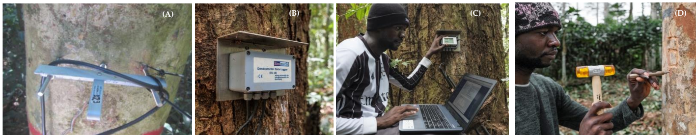
Fig. 1 Radius dendrometer installed on an individual of Pericopsis elata in the Biosphere Reserve of Yangambi (A) and connected to a data logger (B) from where dendrometer growth series can be retrieved (C). Microcores are also collected (D) to assess the monthly pattern of wood formation
