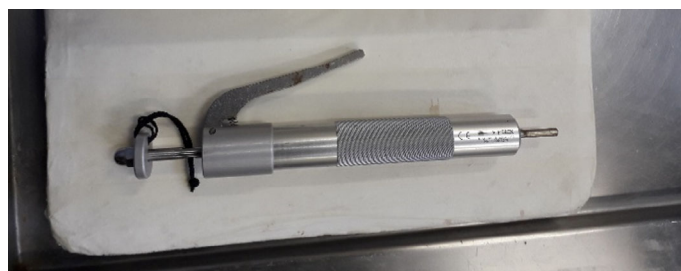
Figure 12: Example of a spring-loaded captive bolt. Source: kindly provided by Velarde A.
