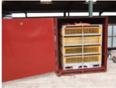
Figure 9: A containerised gassing system. Source: kindly provided by Raj ABM
