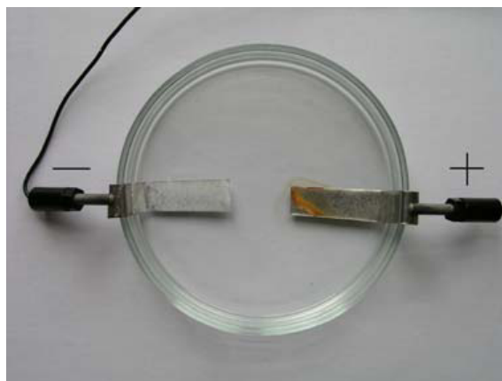
Figure 1. Photograph of the electrolytic cell at the end of the calcium phosphate sedimentation test (in colour online).
