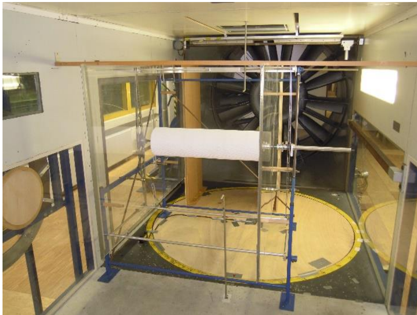
Figure 4.7 Model on balance stand in wind tunnel test section
