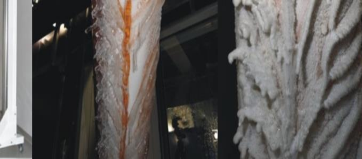
Figure 4.2 Model of structural cable in Climatological section [87]
