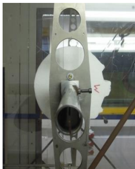
Figure 4.5. "Iced"-model in test section on dynamic balance stand
