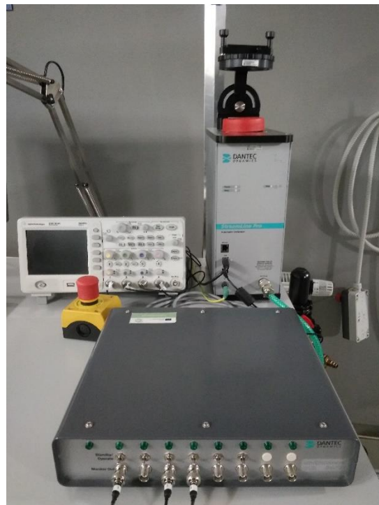
Figure 5.10 Multichannel CTA system by Dantec Dynamics and StreamLine Pro Automatic Directional Calibrator
