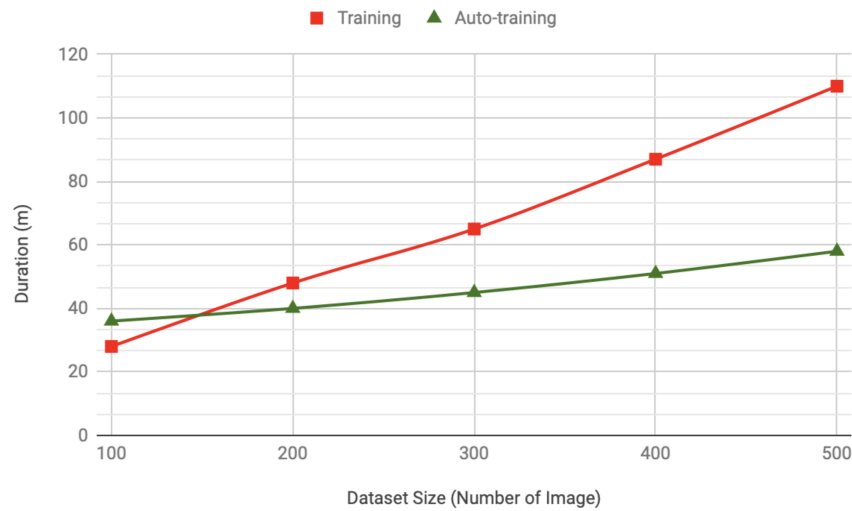
Figure 4.2: Total duration for building a model in Training and Auto-Training Mode (leaf image datasets)
