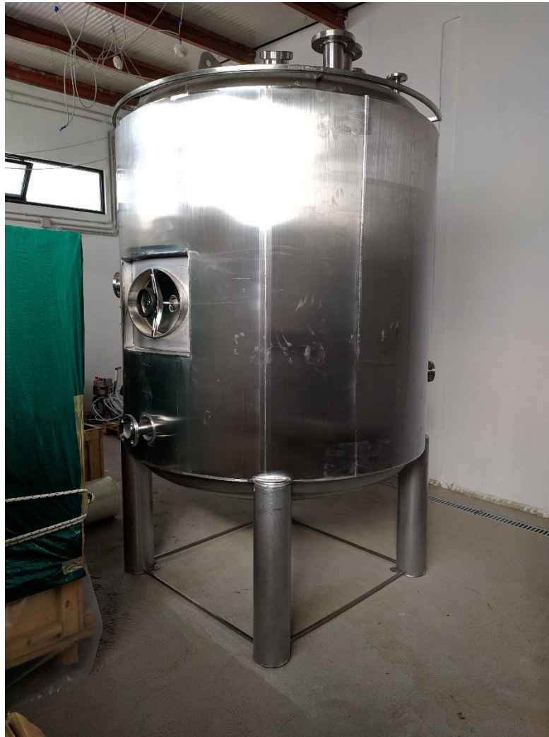
Fig. 114: Detail of the manufactured fermenter designed ad hoc for microalgal heterotrophic cultivation positioned inside the space dedicated to the indoor pilot plant.
