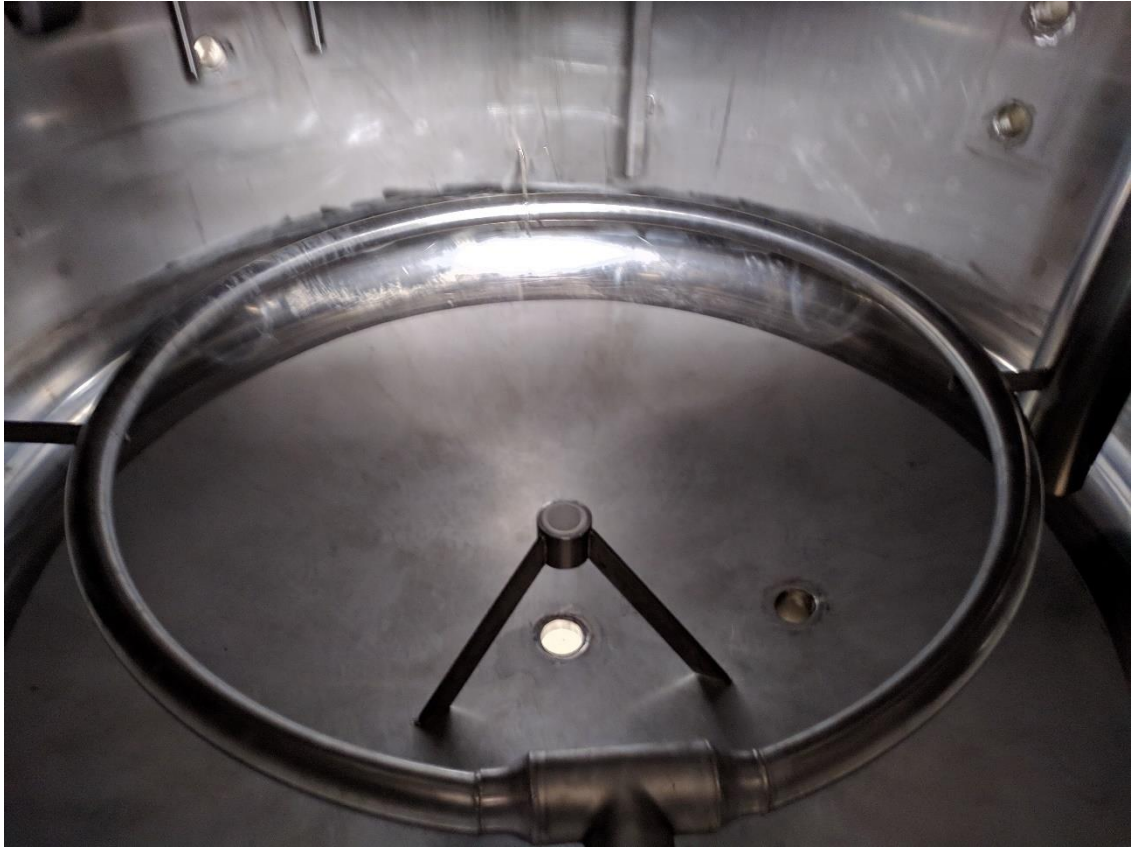
Fig. 110: Detail of the fermenter's sparger designed for the aeration.
