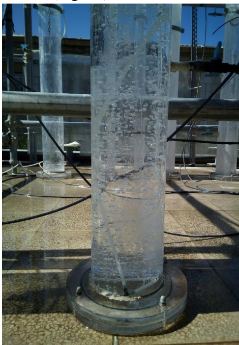
Fig. 44 Toroidal sparger designed and manufactured ad hoc for culture aeration and mixing.
