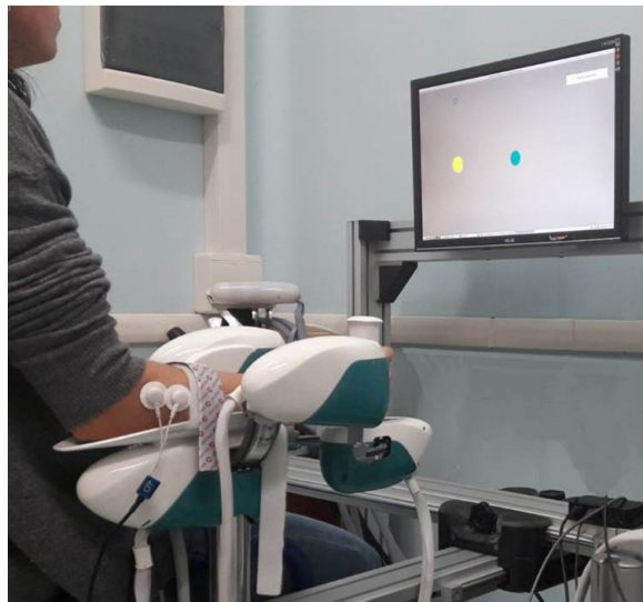
Figure 3.1 Experimental setup. Participant sitting on a chair with the forearm secured to the Wristbot while performing the wrist rotation reaching task. The visual targets of the reaching task are shown on a dedicated screen.
