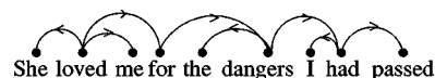
FIG. 1. The syntactic structure of the sentence, “She loved me for the dangers I had passed,” following the conventions in [1]. Here vertices are words and the arcs stand for syntactic dependencies. Following the conventions in [1], arcs go from a head to its modifier. The pronoun “she” and the verb “loved” are syntactically dependent in the sentence. “She” is the modifier of the verbal form “loved,” which is its head. Similarly, the action of “loved” is modified by its object “me.” “Loved” is the root vertex.
