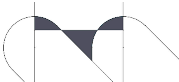
Figure 3. Profile for print orientation angle of 45°, with the areas highlighted in grey.
