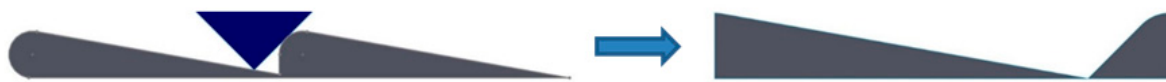
Figure 5. Representation of the roughness tip with the printed layers, for print orientation angle higher than 45^\circ .
