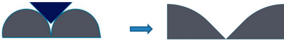
Figure 4. Schematic of the printed layers with the roughness tip, for print orientation angles higher than 45^\circ .
