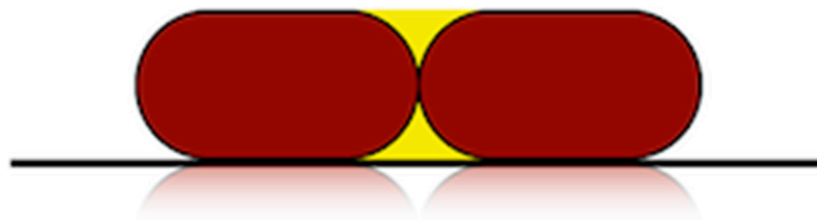
Figure 1. Schematic of the cross-section of two adjacent deposited filaments with print orientation angle of 0^\circ (the horizontal line corresponds to the printing bed).
