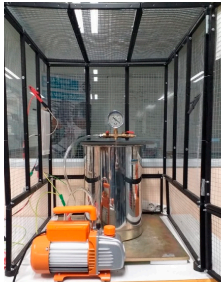
Figure 3. Low-pressure chamber and vacuum pump used for the experiments.
