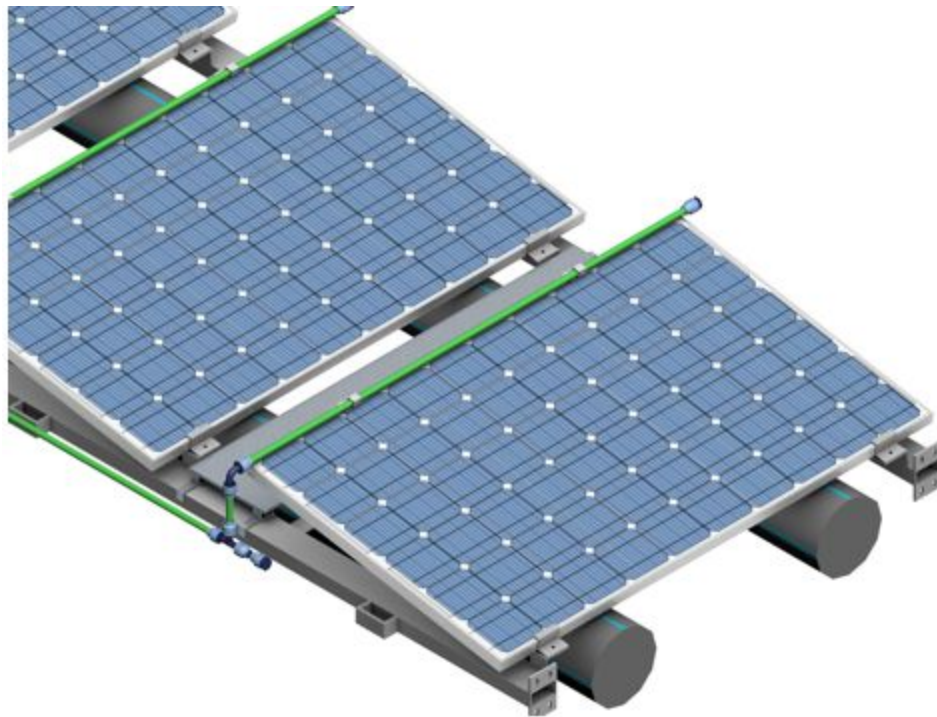
Figure 21. Diagram of a WVC system (Rosa-Clot M., Tina G. M., 2018)
