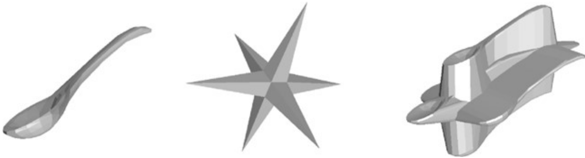
Figure 4: Minkowski sum of a spoon and a star (image courtesy of Peter Hachenberger and the CGAL project).
