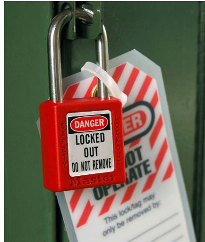
Figure 3.1. ECPL compliant padlock locking equipment. Source: [4]
