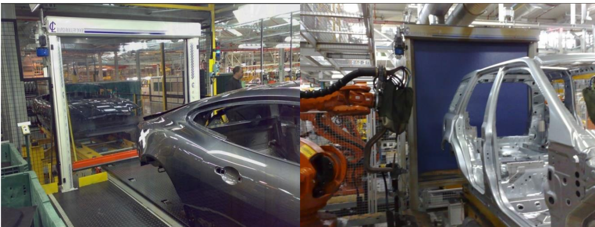
Figure 3.3. Rapid Roller Door. Open in the left image and closed in the right. Source: Centreline Machine Guards LTD. Source: [6]
