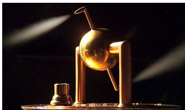
Figure 1.1: Replica of Hero's aeolipile [4]
