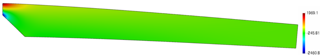
Figure 7.4: Deformed configuration ( \times 1000 ) and \sigma_{\zeta\zeta} (KPa) of the blade for the moment of maximum stress.
