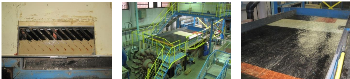
Figure 4. Reproduction of C3 clogging pattern for the Barcelona inlet, and views of the experimental set-up
