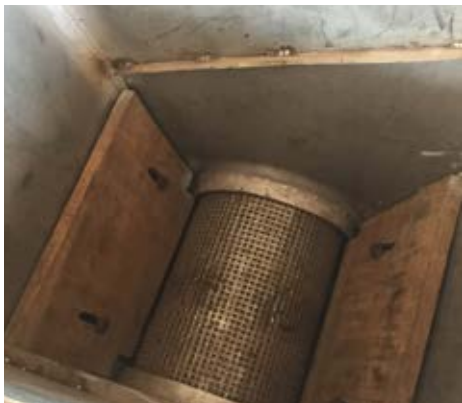
Figure 3: Rasper with wooden block (Photo: ILRI/Tunde Amole)
