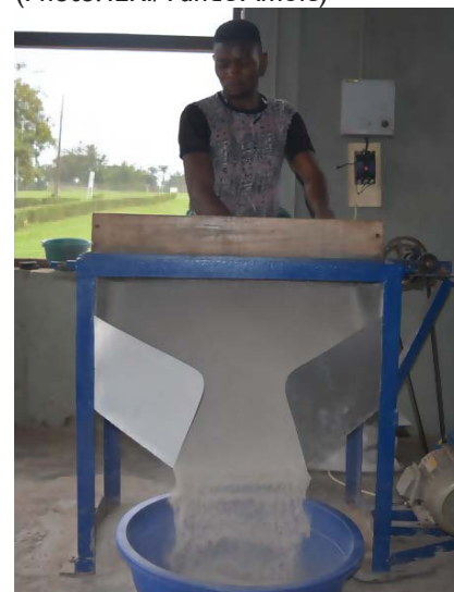
Figure 6: Sieving pulverized cassava peel with a mechanical sieve (Photo: ILRI/Tunde Amole)
