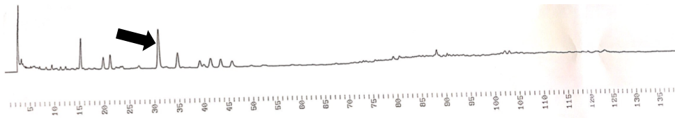
Fig.3 HPLC chromatogram of a decoction of medical-grade agarwood Black arrow: Agarotetrol peak
