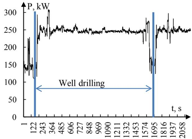
Figure 2: Relation diagram  $P=f(t)$  for DM-H drilling rig
