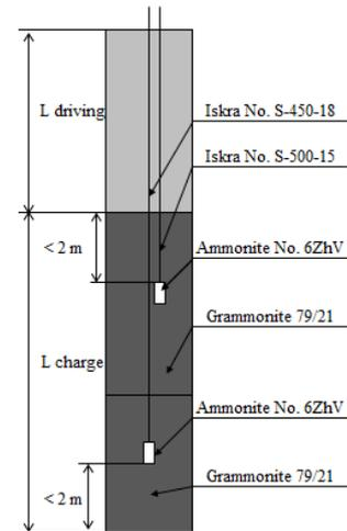
**Figure 4.** Standard composition of the blasthole charge for hard blasted rocks ("Iskra" No. S-450-18 — 1 unit, "Iskra" No. S-500-15 — 1 unit, Ammonite No. 6ZhV — 6 kg, cartridge of 2.85 kg, Grammonite 79/21 — 864 kg)
