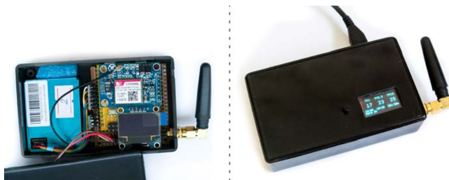
Figure 1. Prototype of the device for measuring the level of the atmospheric pollution by particulate matter.
