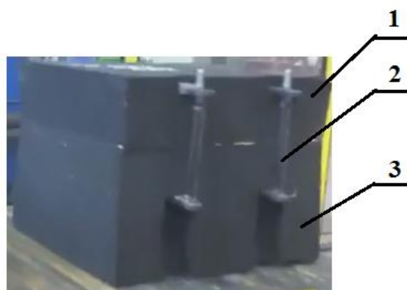
Fig. 2. Complete mold, form made on \alpha -set to process: 1 – Top half-mold; 2 – Mechanical fastening of half-molds; 3 – Bottom half-mold
