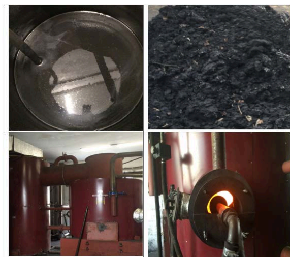
Fig. 3. WCS from the filter cake and the burning process of the fuel.
