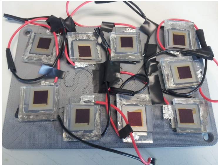
Figure 6.3: Nine DSSCs with 1 cm 2 photoactive areas soldered in series to provide a 5.4 V operating voltage, and an open circuit voltage of 7.2 V.
