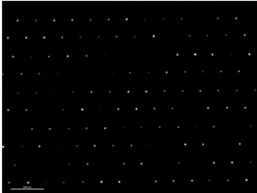
Figure 3.21: Light transmission image of in-house laser perforated Ti foil with 20 % laser power. Some voids were perforated, while many of the voids in the foil remained unperforated
