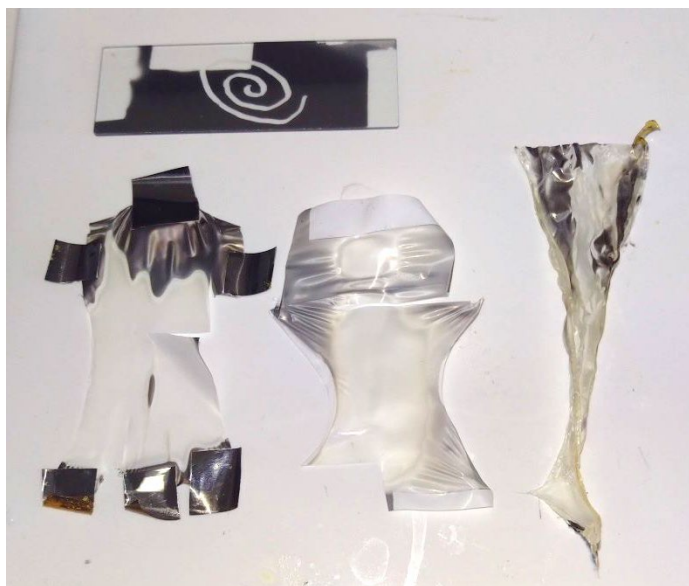
Figure 3.50: Ti thermally deposited onto Celgard and a microscope slide. The microscope slide has a reflective metallic coating. Wrinkled and opaque sections of the Celgard are no longer porous due to thermal damage. The metallised sections of the Celgard are reflective but may be thermally damaged.
