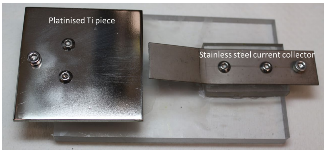
Figure 4.13: Image of the open cell holder with platinised Ti counter electrode and stainless steel current collector with upwards bend to connect to the photoanode.
