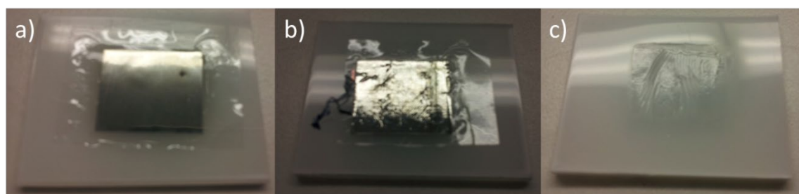
Figure 3.34: Ti foil adhered to polypropylene with Surlyn thermoplastic. a) 25 \mu\text{m} Ti foil adhered with a flat surface, b) 5 \mu\text{m} Ti foil adhered with a wrinkled surface and c) indentations present on the polypropylene following delamination of the Surlyn/Ti foil.
