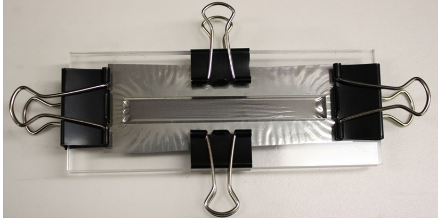
Figure 3.27: Laser perforated 25 \mu\text{m} Ti foil sandwiched between a Perspex jig. The perforated area is 8x80 mm in size with voids 20 \mu\text{m} in diameter every 50 \mu\text{m} .
