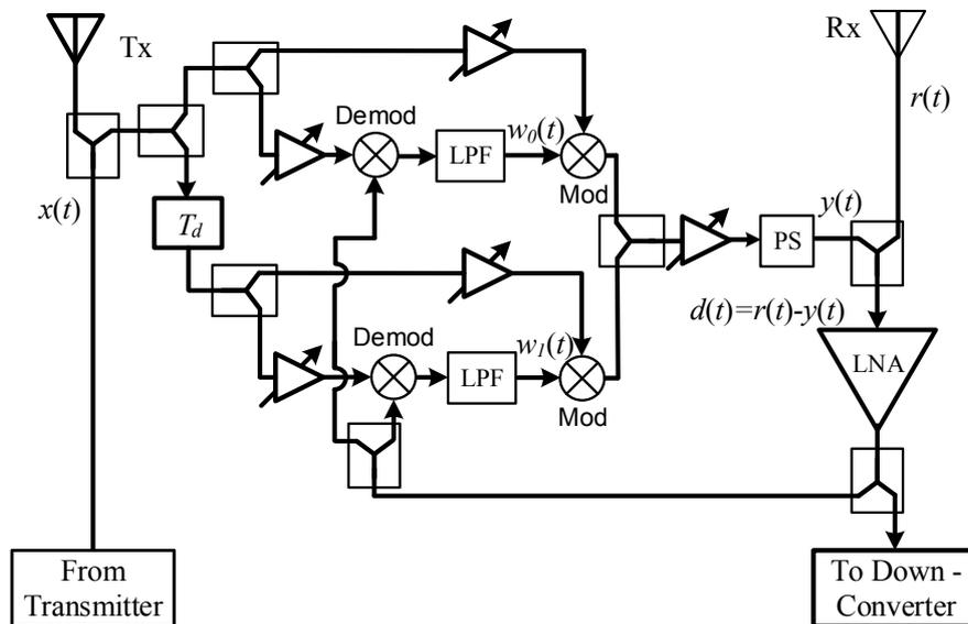
**Figure 4.** A practical structure of the ALMS loop.
