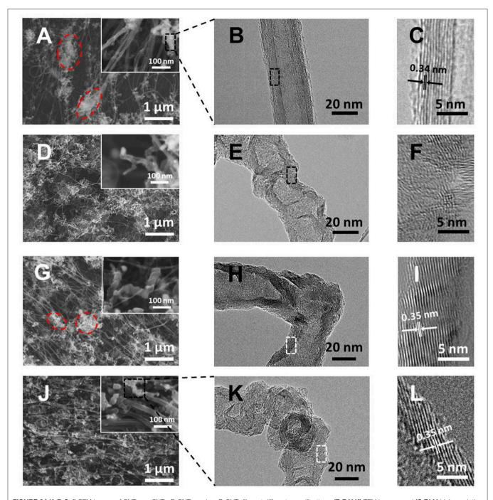
FIGURE 2 | (A,D,G,J) SEM images of CNTs, py-CNTs, B-CNTs, and py-B-CNTs films at different magnifications; (B,E,H,K) TEM images; and (C,F,I,L) high-resolution TEM images of CNTs, py-CNTs, B-CNTs films, respectively.
