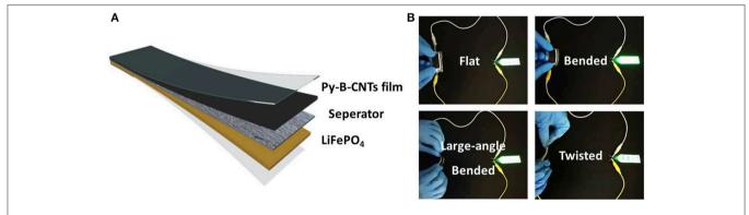
FIGURE 5 | (A) Schematic illustration of the flexible LIB with py-B-CNTs film and commercial LiFePO<sub>4</sub> as electrodes; (B) photographs of the flexible LIB powering a light-emitting diode board under various bending conditions.
