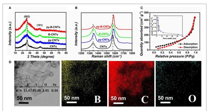
FIGURE 3 | (A) XRD patterns and (B) Raman spectra of the samples; (C) nitrogen adsorption/desorption isotherms with the pore-size distribution (inset) of py-B-CNTs film; (D) the EDS elemental analysis of py-B-CNTs and corresponding elemental mapping of the region.
