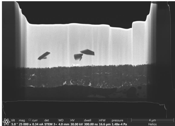
Figure A- 3: SEM image of thin lamellar extracted from the ball scar after lubrication test
