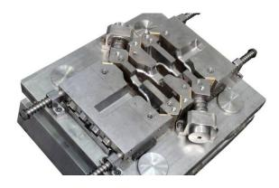
This tool can typically be used in normal eccentric presses to produce work pieces.
