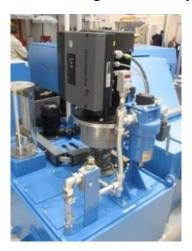
As regards energy efficiency and costs, the flow rate and pressure have to be optimised. In a specific case, the optimum pressure and flow rate were 15 MPa and 31 l/min, respectively. The cleaning efficiency is influenced by the nozzle design, the orifice area and the jet opening angle (Brinksmeier et al., 2015).
