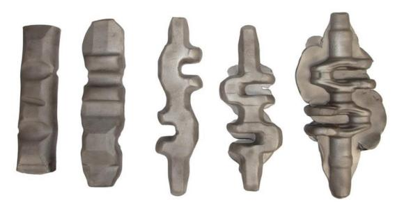
In order to minimise the formation of flash, the complete forging concept, including the forging tools for all the different steps have to be adapted. In the initial forging steps, traditional forging set-up is replaced by "flash free" as shown in Figure 4.26.
