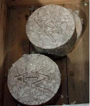
Most briquetting presses are suitable for processing various kinds of swarf resulting from machining of steel, cast iron, stainless steel, aluminium, etc. (keeping in mind the need to avoid contamination if the same machine is used for different streams) and are available in different sizes and filling variants to suit the specific needs of manufacturers and input material. Briquetting can be carried out in-house or outsourced.
