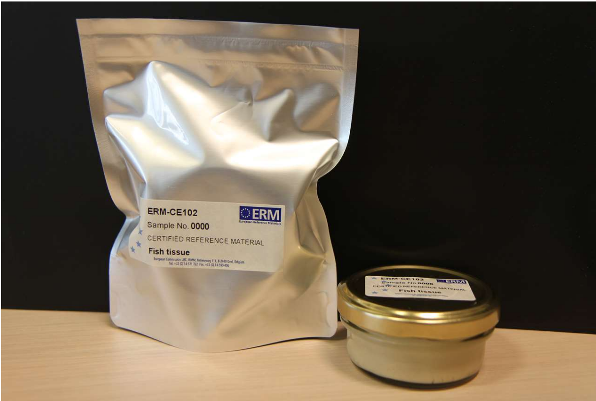
Figure 2: Example of ERM-CE102 unit: jar filled with fish paste and its protective pouch
