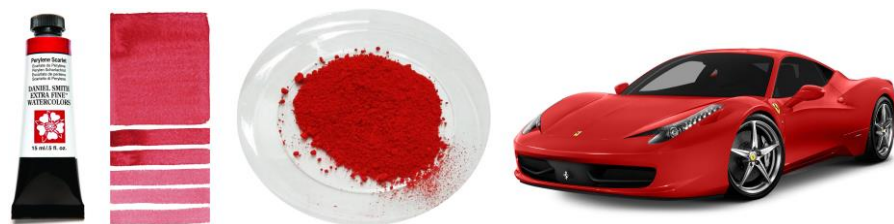
Figure 2.5. Due to their intense red color, perylenes belong to the most important class of paints (left), pigments (center) and coatings (right) for industrial applications. [107]
