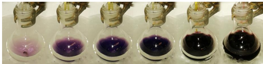
Figure 5.4. Porphyrin synthesis: color change upon dropwise addition of dicarbinol 11 and dipyrromethane 7 .
