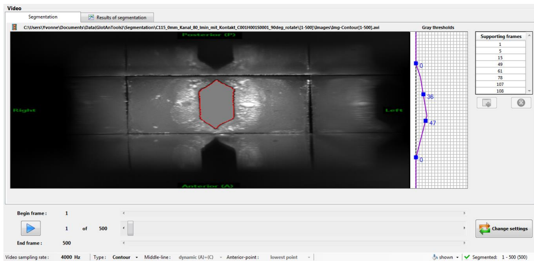
A Figure 97 - Model C115 in 18mm channel configuration in M2 during the setting of the maximum glottal gap with seatpoints with GAT.
