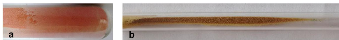
Figure 7. 2-trifluoromethylbiphenyl 1 deposited on activated aluminium oxide: a) at the room temperature; b) at 200 °C for 10 min. Adapted with permission from O. Papaianina and K. Yu. Amsharov, Chem. Commun. , 2016 , 52, 1505. DOI: 10.1039/C5CC08747 Copyright 2016 The Royal Society of Chemistry.
