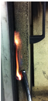
Fig 9. Testing leaked gases
