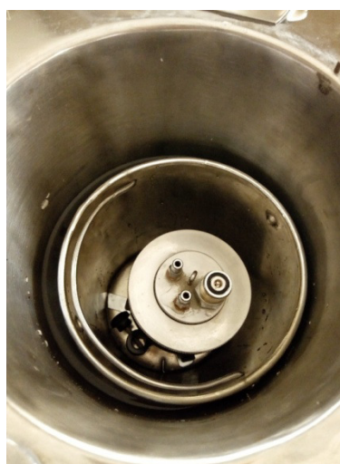
Plate 6. Bomb vessel placed inside calorimeter vessel
