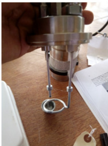
Plate 4. Bomb Electrode slots to accept the use of screw microchrome wire.
