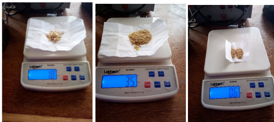
Plate 2. Labtech BL20001 Electronic Compact Scale measuring the mass of Biomass.
