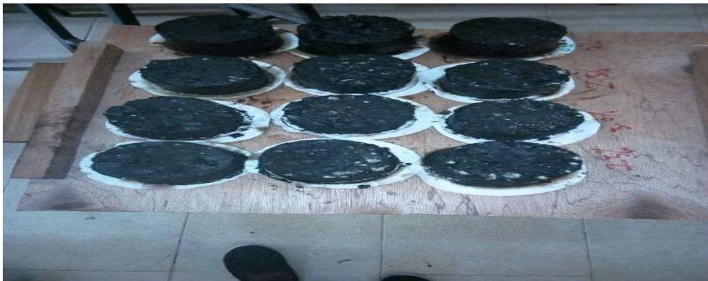
Figure 2. Samples of compacted modified specimen
