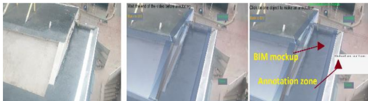
Fig. 3. From left to right: a) video of the building from a drone, b) MR visualisation: superimposition of the video and the BIM model c) MR interaction: annotations [20]
