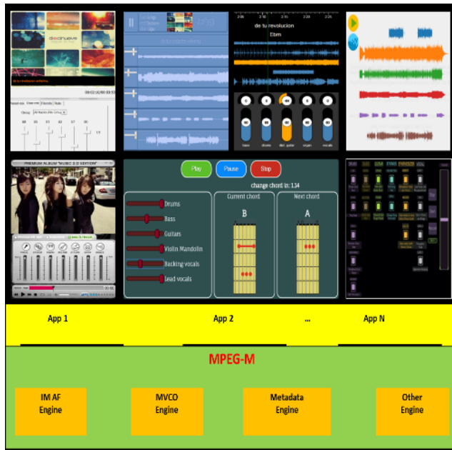
Figure 2. MPEG-M architecture adapted for enabling interactive music applications and services with IP rights tracking.
