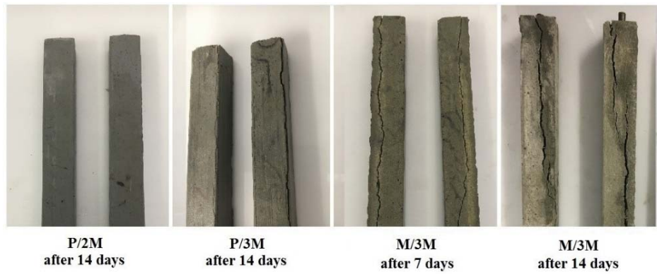
Fig. 5 Photographs of 25 x 25 x 285 mm geopolymer paste or mortar prisms stored at 80°C in NaOH solutions of different concentrations: P/2M - pastes stored in 2M NaOH, P/3M - pastes stored in 3M NaOH, M/3M - mortars stored in 3M NaOH.
