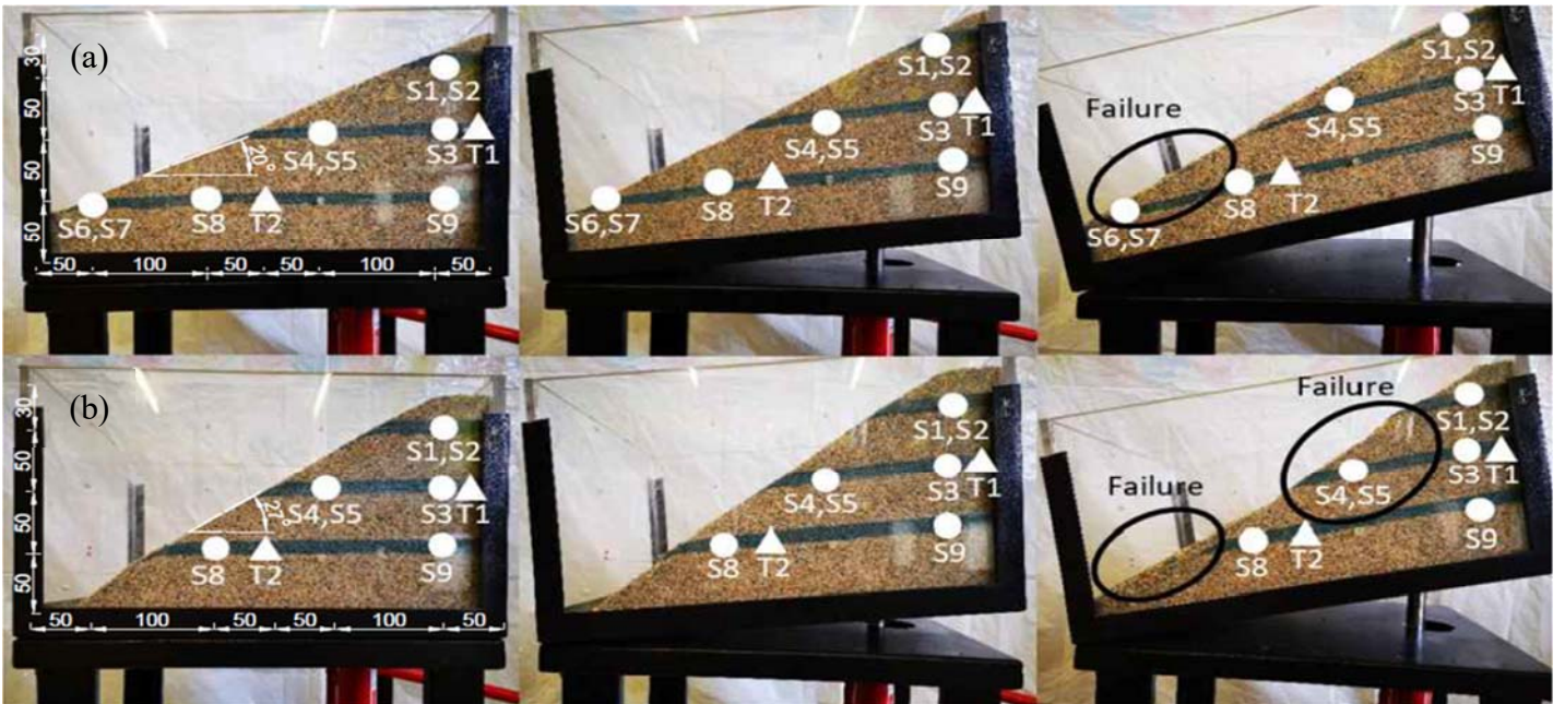
Figure 4. Model geometries for (a) Test 1 and test 3 (b) Test 2 and test 4. This picture also depicts the FBG sensor layout for (a) Test 3 (b) Test 4.
