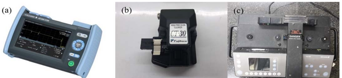
Figure 2. The system needed to create hetero-core sensors and monitor them. The system needed is: (a) Yokogawa AQ1000 OTDR (b) High precision cleaver (c) FSU 925 Fusion Splicer.
