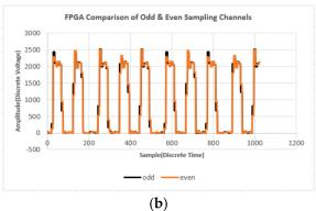
**Figure 9.** FPGA architecture implementation results: (a) Source signal which is in phase with I and odd/even order sampling results; (b) Odd and even order sampling results with Vivado integrated logic analyzer (ILA) window configured to 1 kilobyte.
