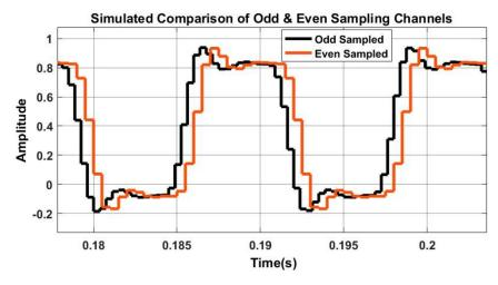
Figure 2. This portrays the phase lag performance between odd and even order sampling. Odd order sampling is marked by black and even order sampling is marked by red. It should be noted that the (n-1) phase lag between even order sampling (red) and odd order sampling (black) varies per period interval.
