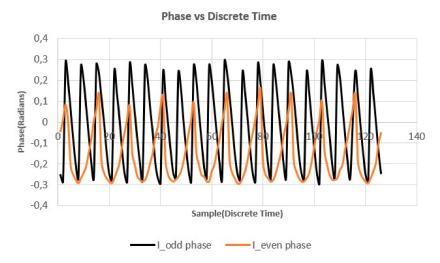
Figure 7. The phase error behavior of the new odd/even order sampling.
